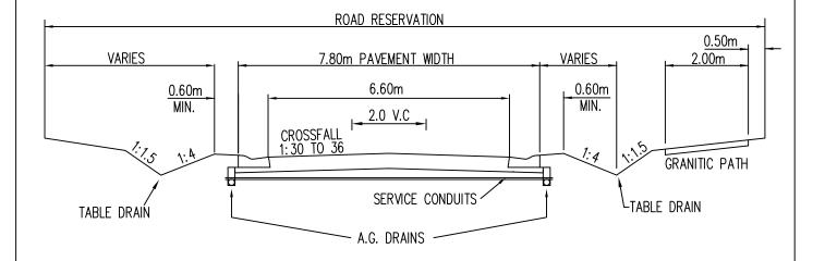
TYPICAL CROSS SECTION FOR HIGH SPEED RURAL ROADS (WITH CONCRETE KERB AND CHANNEL)
