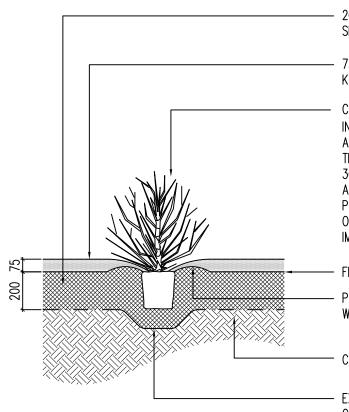
200MM DEPTH INSITU OR IMPORTED TOPSOIL, AS SPECIFIED
